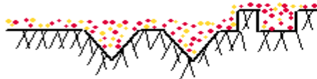
Water evaporates but a layer of dirt and dried detergent mixture remains, and the build-up process begins.
